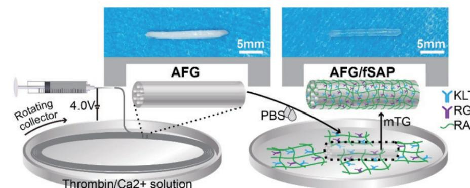
Diagram of AFG/fSAP synthesis process
