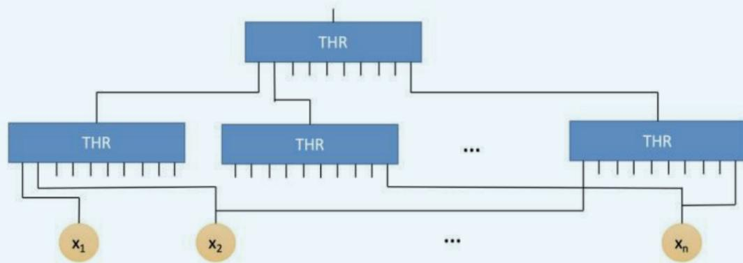
A depth-2 linear threshold circuit
