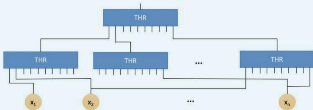
A depth-2 linear threshold circuit
