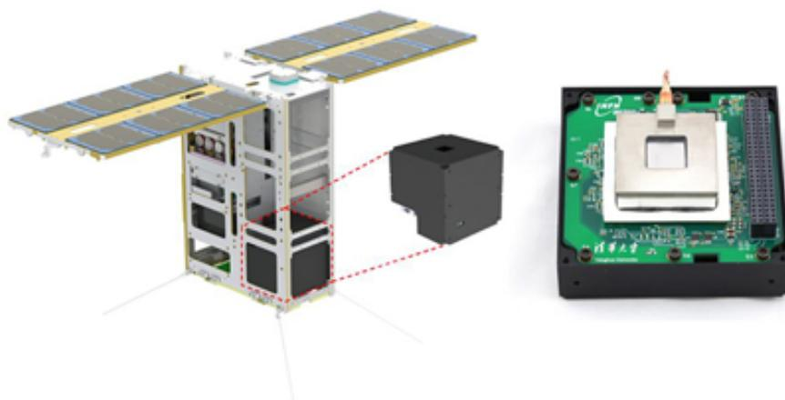
Figure 1. The PolarLight detector and the CubeSat.
