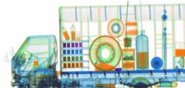
The comparison between single-energy grayscale image and dual-energy color image with the patented recognizing technology
